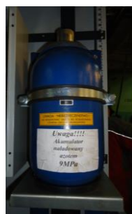
→ Hydraulic Accumulator for Emergency Fast Operations
